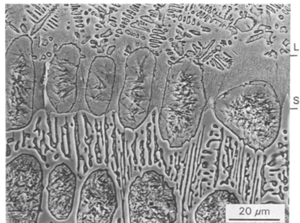
Figure 7 Detail of the "mushy zone"—transition between the melted and austenitized zones, v = 8.5 \text{ cm s}^{-1} , SEM. L ... liquidus, S ... solidus \approx T_E = 1150^\circ\text{C} .
